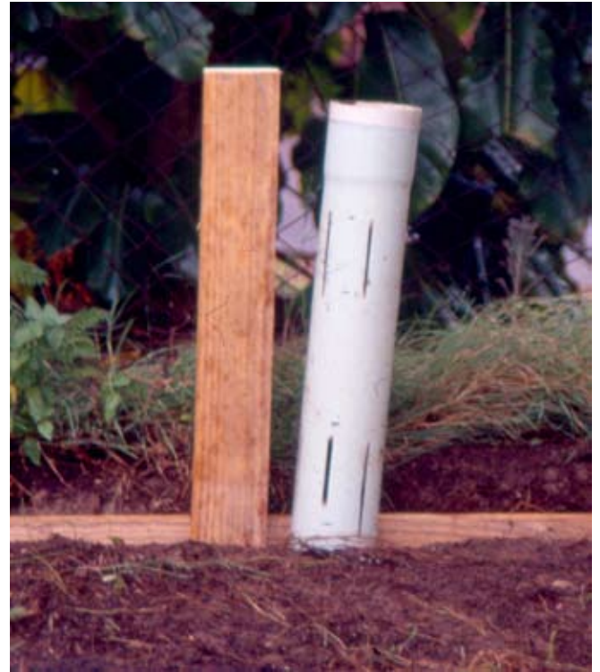
Figure 4. Termite aggregation station with slotted, PVC stormwater pipe and timber before installation.
